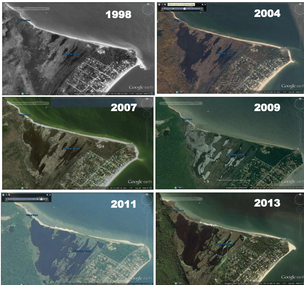
Figure 7. Google Earth images of Cove Point marsh from 1998 to 2013. The restoration project and breakwaters can be seen in the 2011 and 2013 photographs.
