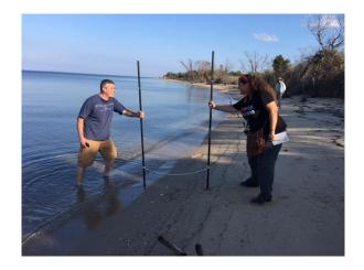
Figure 3. Eric Fons and Dimitra Neonakis showing the use of Emery rods on a downward sloping beach.
